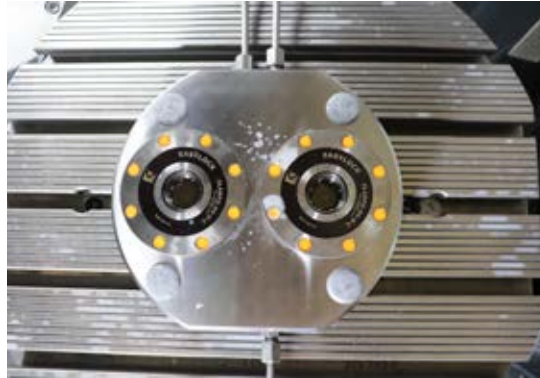
Upper table for automation system
