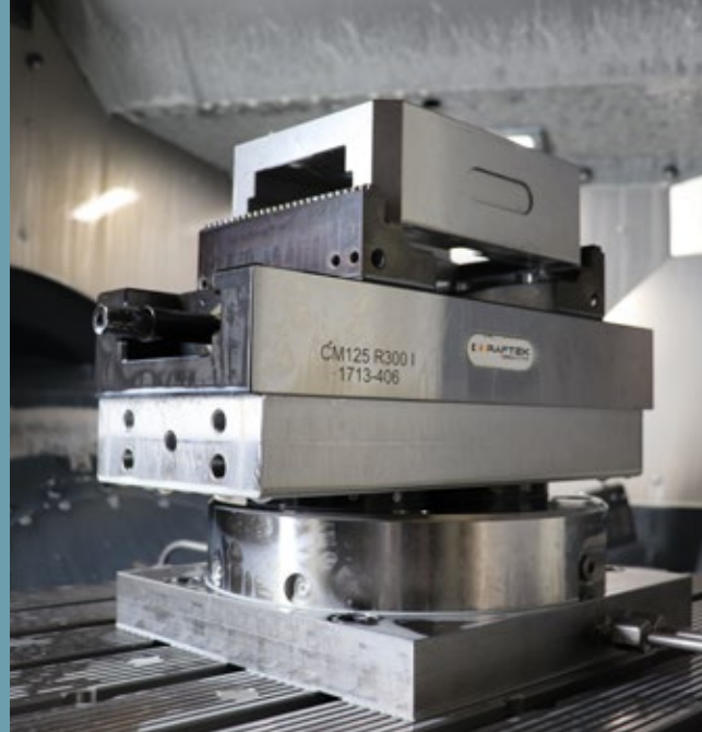
Upper table with EASYLOCK zero point systems using an adaptor plate.
