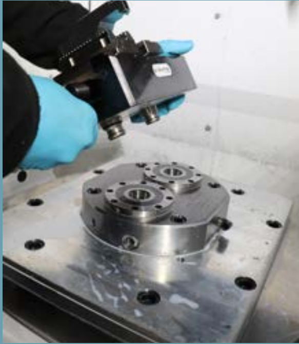
Mounting of an EASYCLAMP vice with clamping pins over an upper table equipped with our EASYLOCK zero point systems.
