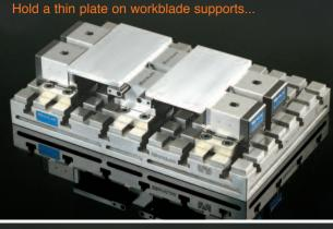
Clamp two medium sized parts by ganging laws together using the double-sided sideclamps
