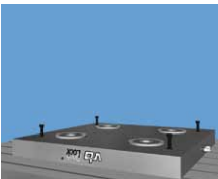
Mount combination plate to machine-tool table
